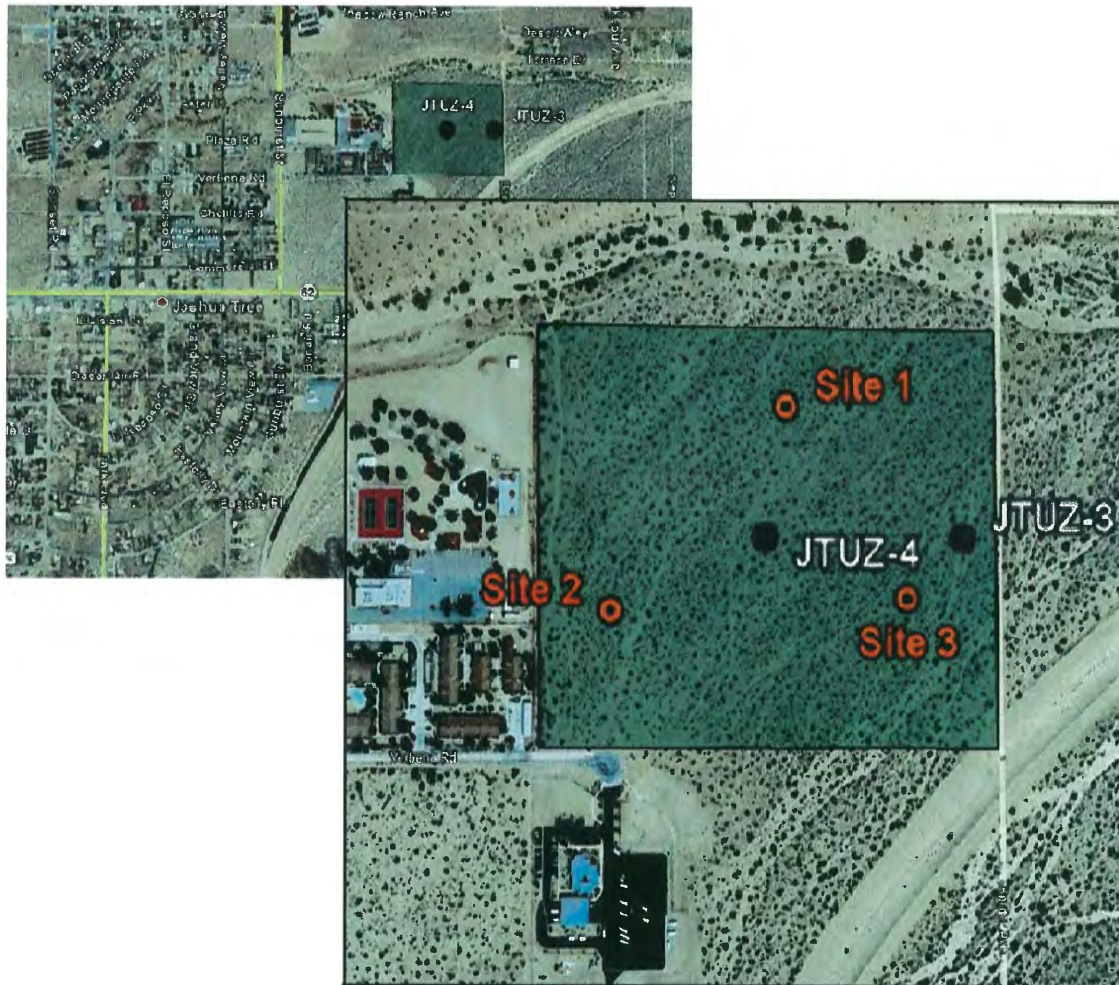
Figure 3. Infiltrimeter test site locations, USGS boreholes JTUZ-3 and JTUZ-4, and the area under consideration for artificial recharge sites, Joshua Tree, California.
